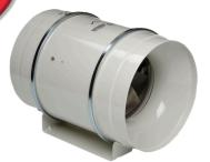
Low profile mixed flow fans, manufactured in plastic material (up to model 150) or in galvanized steel sheet protected with Epoxy paint (models 200, 250, 315, 355, and 400), with external terminal box, removable motor-impeller assembly and adjustable single-phase motor, Class B. IP44.
